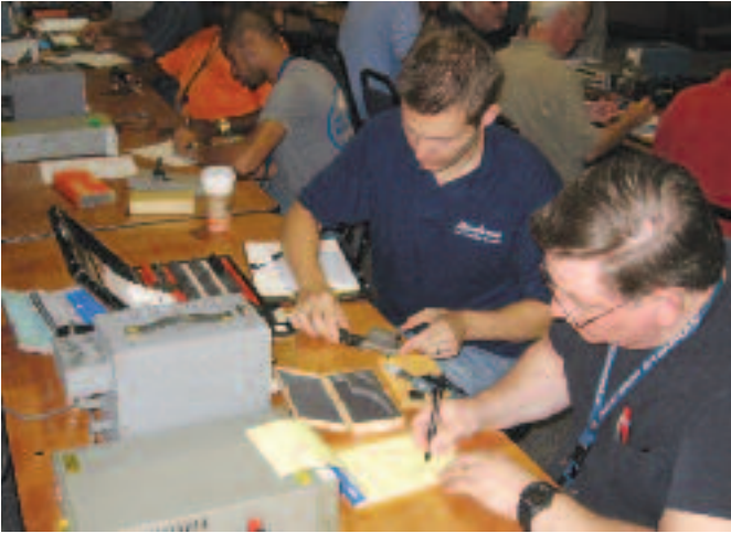
Foreground: Henry Zumbrun uses Digital Calipers to measure a Gage Block while Bill Brown records the measurement result.
