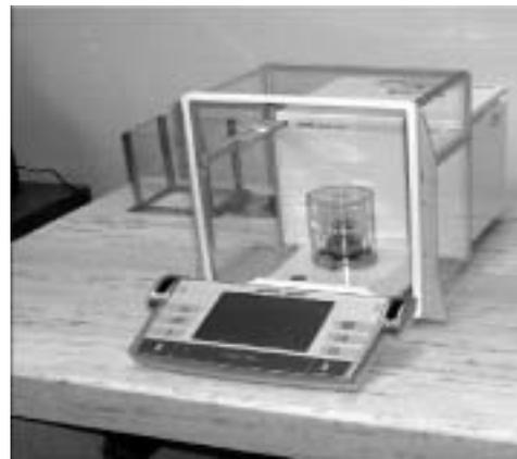
Figure 3: Setup used to weigh 10mg samples with an evaporation trap.
