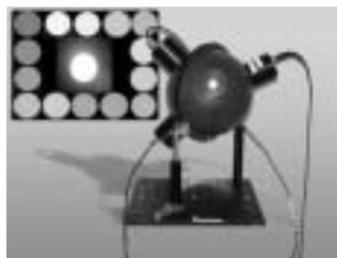
*NIST's new portable "rainbow" source for calibrating color measurement instruments. In the background are a sampling of colors generated with the source. Photo courtesy National Institute of Standards and Technology.*
